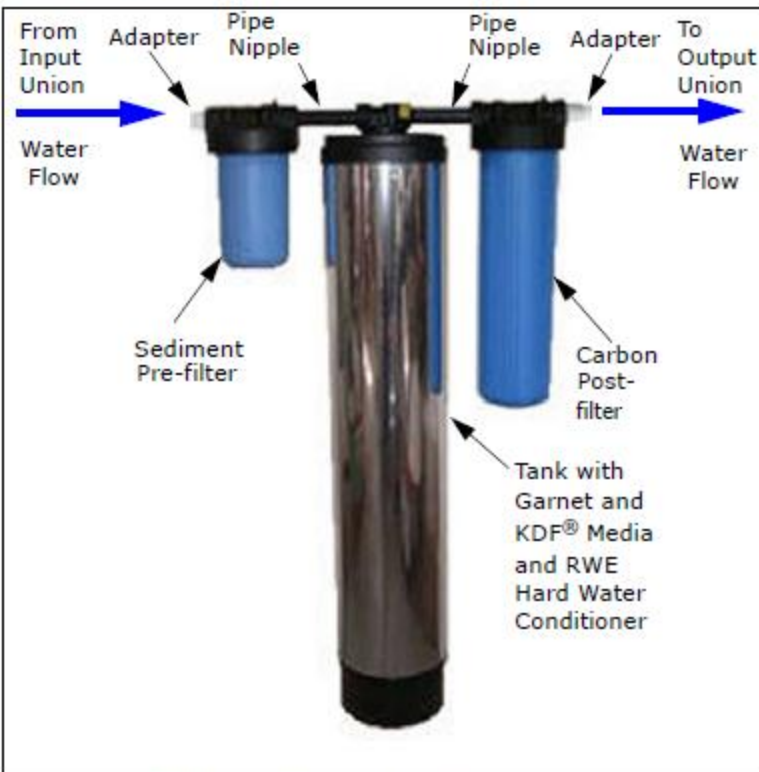
Figure 10 Total Water Filtration System
